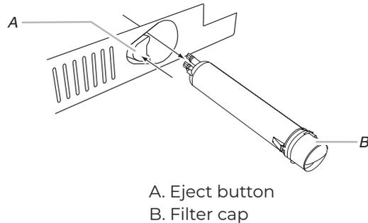
2. Remove the cap by turning it counterclockwise until it stops.
