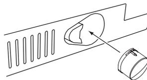
4. Turn the cap counterclockwise until the cap slips into the attachment slot. Then, turn the cap clockwise until it is in a horizontal position.
