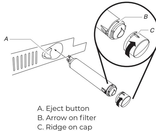
6. Push the new filter into the opening in the base grille. As the filter is inserted, the eject button will depress. The eject button will pop back out when the filter is fully engaged.
