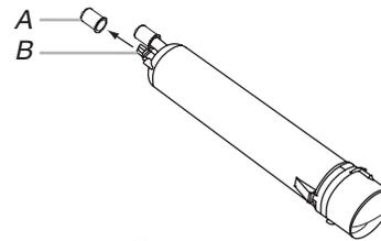
4. Remove the covers from the O-rings. Be sure the O-rings are still in place after the covers are removed.
